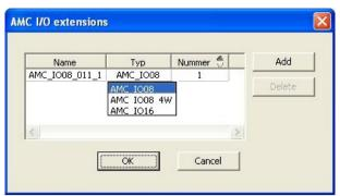
The list entry AMC2 4W can only be added only once, whereas up to three I/O Extensions can be added.
