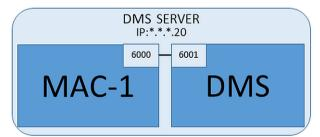
For a minimal system configuration one MAC is required. In this case the MAC can reside on the DMS server.
