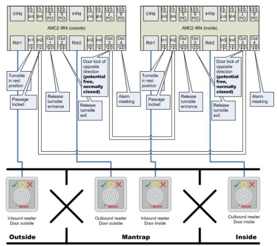
Connections to the door locks for the opposite direction ensure that only one of the turnstiles can be opened at any one time.
