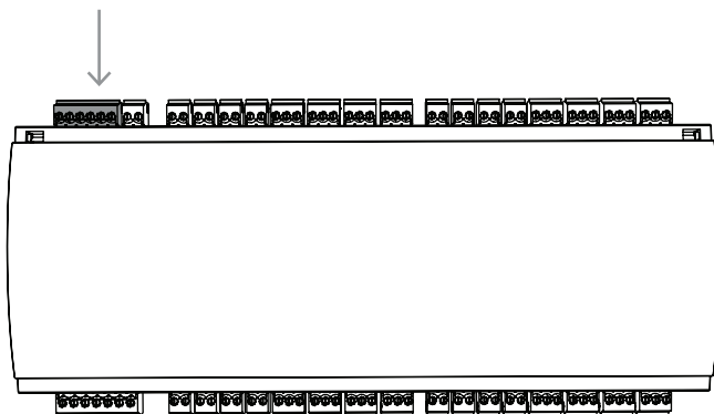
Figure 4.9: Location of the RS-485 extension module bus
