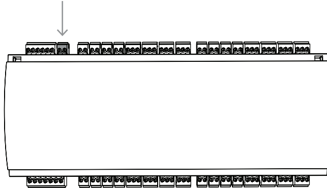
Figure 4.18: Location of the tamper protection contact
