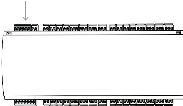
Figure 4.7: Interface for internal power supply
