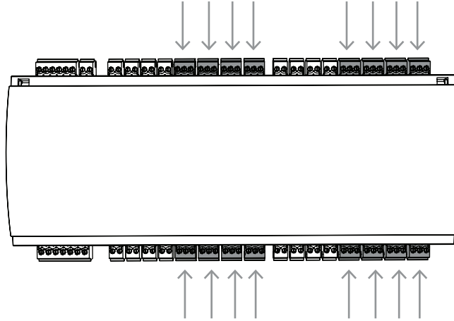
Figure 4.12: Location of the relay output connectors
