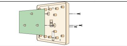
Install the cover tamper screw. Refer to illustration below.
