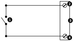
Figure 14.3: N.O. - Normally Open Non-supervised Connections
