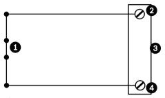
Figure 14.4: N.C. Normally Closed Non-supervised Connections
