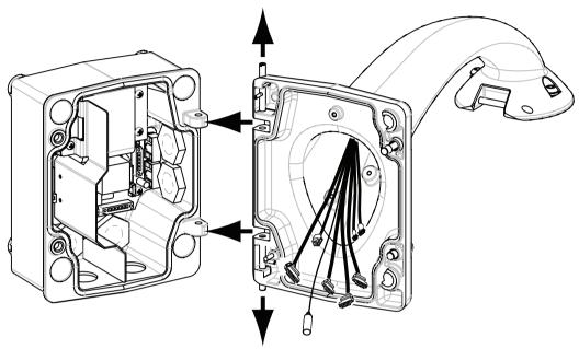
Figure 10.7: Pendant Arm to Power Box Hinge Alignment
