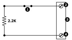
Figure 14.2: N.C.S. - Normally Closed Supervised Connections
