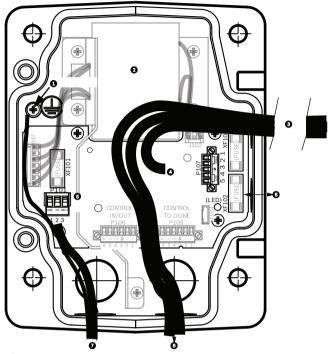
Figure 11.3: Power Supply Box Connections
