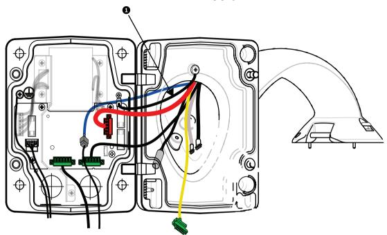
Figure 10.8: Pendant Arm connections to Power Supply Box
