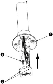
Figure 11.8: Pipe Interface Board to Dome Cap Assembly
