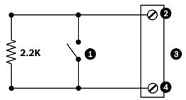
Figure 14.1: N.O.S. - Normally Open Supervised Connections
