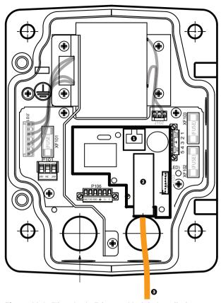
Figure 11.2: Fiber Optic Ethernet Module installed
