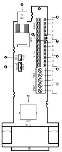
Figure 11.6: Pipe Interface Board Connections
