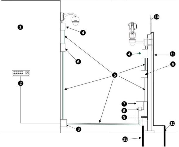
Figure 5.1: Correct outdoor installation with proper surge/lightning suppression
