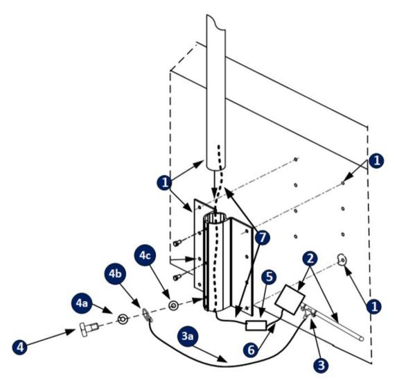
Figure 5.2: Grounding a parapet mount
