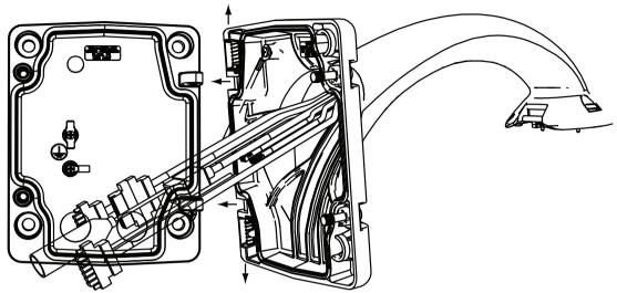
Figure 10.9: Connect Pendant Arm to Mounting Plate
