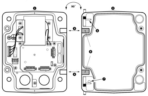
Figure 11.4: Align Cover Door Hinge to Power Box
