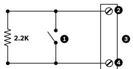
Figure 10.2: N.O.S. - Normally Open Supervised Connections
