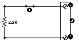
Figure 10.3: N.C.S. - Normally Closed Supervised Connections
