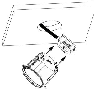
Figure 7.5: Attach Housing to Interface Box
