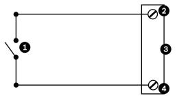
Figure 10.4: N.O. - Normally Open Non-supervised Connections
