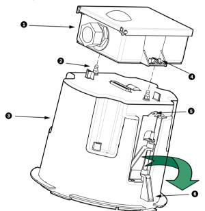
Figure 7.6: In-Ceiling Housing and Interface Box
