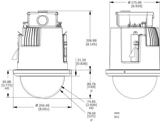
Figure 7.1: AUTODOME 7000 Dimensions – In-ceiling
