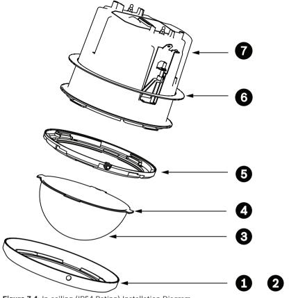
Figure 7.4: In-ceiling (IP54 Rating) Installation Diagram
