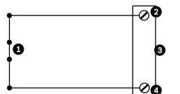
Figure 10.5: N.C. Normally Closed Non-supervised Connections
