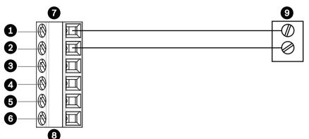
Figure 10.6: Connections for audio over an Ethernet network
