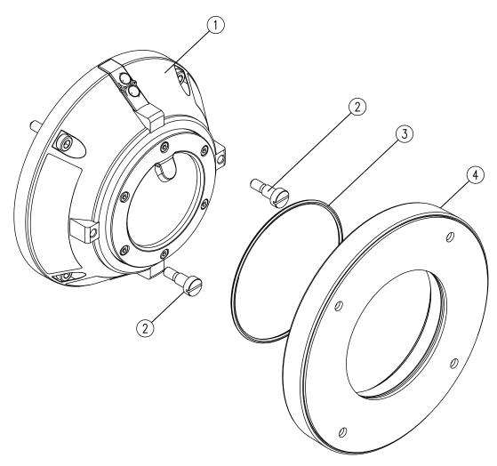
Fig. 20: FMX5000 IR Ex bracket mount installation
