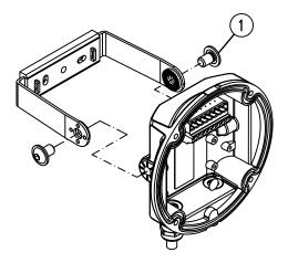
Fig. 15: MX5000 Ex detector base for bracket mounting
