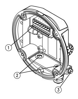
Fig. 16: MX5000 Ex detector base
