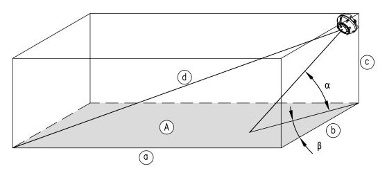
Fig. 11: Room monitoring as per VdS 2095: 2010-05 (07)
