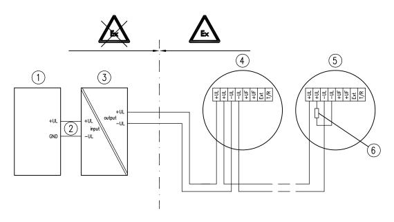
Fig. 25: Alarm line wiring without a fault line with a galvanically isolated barrier
