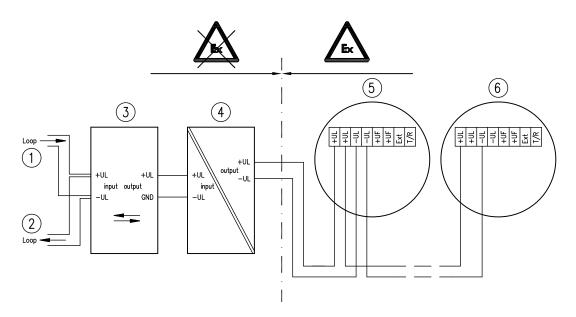
Fig. 30: Wiring diagram – individually addressable operation in the spur at the loop
