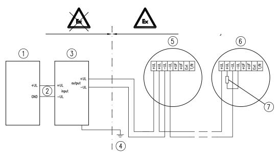
Fig. 24: Alarm line wiring without a fault line with a zener barrier
