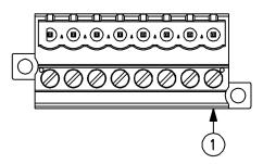
*Fig. 5: Detector base connecting terminal*
