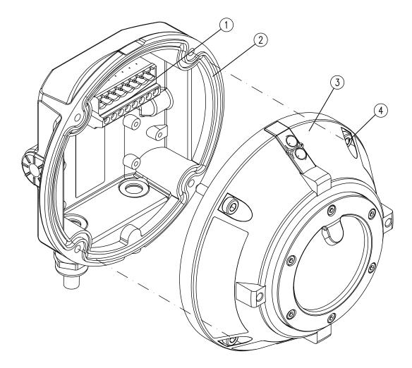
Fig. 17: Screw the FMX5000 IR Ex to the detector base
