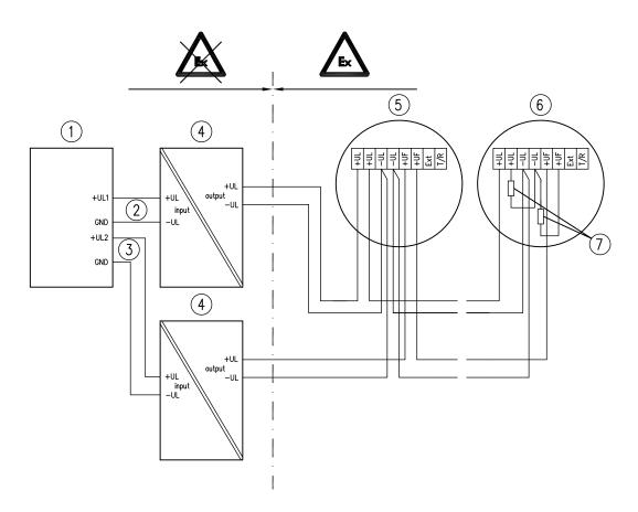
Fig. 27: Alarm line wiring with a fault line and a galvanically isolated barrier
