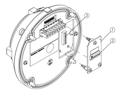
Fig. 31: Mount the KMX5000 AP Ex communication module on the detector
