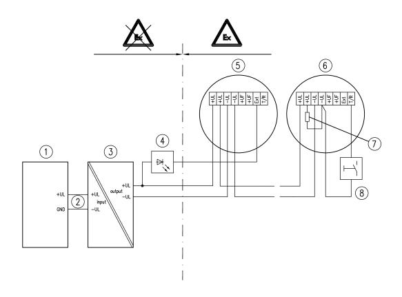
*Fig. 29: Alarm line wiring, external indicator and test/reset button with a galvanically isolated barrier*
