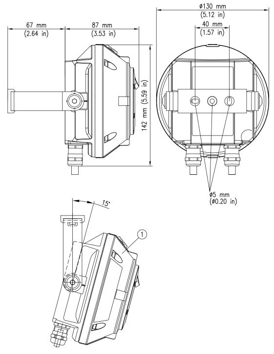
*Fig. 14: FMX5000 IR Ex – Device and assembly dimensions and bracket mounting inclination angle*
