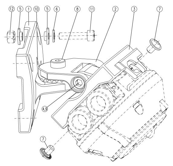
Fig. 19: Assembly of MX5000 ST wall mounting bracket
