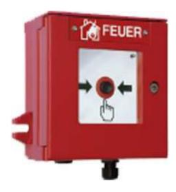
The call points are used to manually activate the alarm in zones 1, 2, 21 and 22 at risk of explosion. They are encapsulated, intrinsically safe and do not require any safety barriers.
