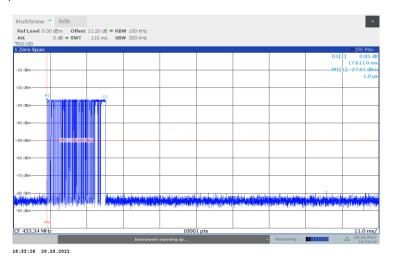
Figure 8.6-2: Transmission pulse
